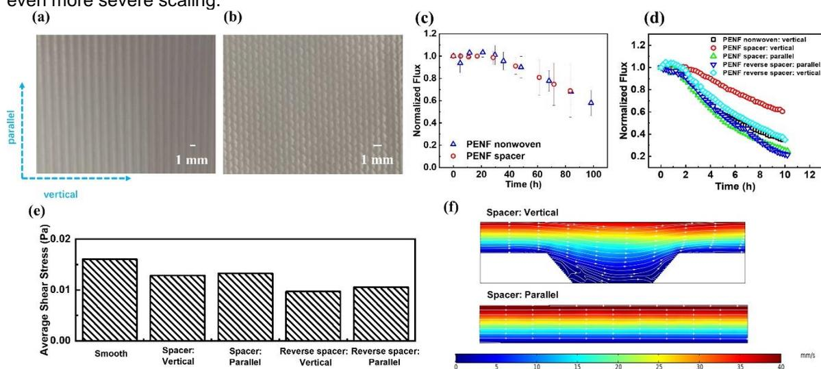
**Figure 3.** (a)-(b) photos of the surfaces of (a) spacer-imprinted PENF membrane; (b) reverse spacer-imprinted PENF membrane. (c)-(d) normalized flux of (c) dead-end scaling; (d) crossflow scaling. (e) Average shear stress on smooth surface and PENF on spacers of different configurations. (f) streamline profiles on PENF imprinted by permeate spacer.
